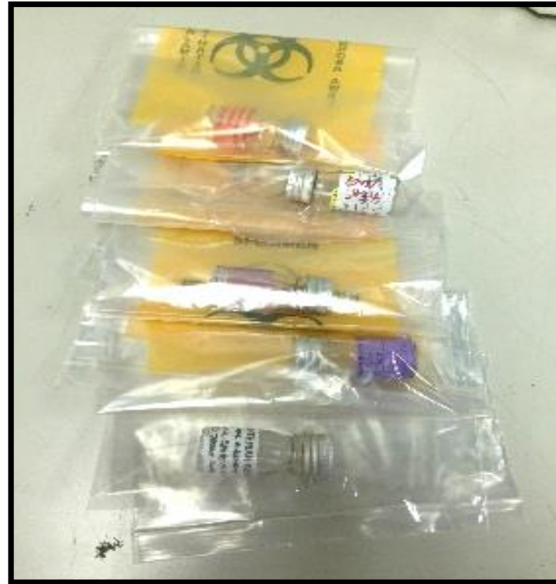
Secondary receptacle watertight, leak-proof biohazard plastic bag
