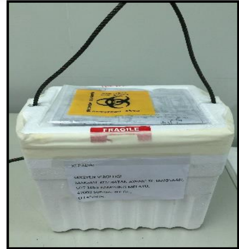
Outer packaging Rigid Outer box, recommended Styrofoam
