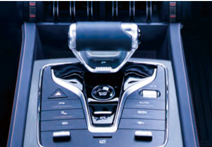
Push-type Electronic Gear Lever
